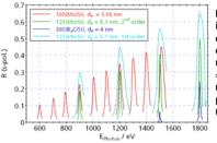
Reflectance steadily increases with photon energy up to absorption edges of the multilayer materials. => Tungsten based multilayers only useful for photon energies ≤ 1.5 keV (Al emission line).
